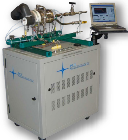
Fuel Reformer Test Cart
