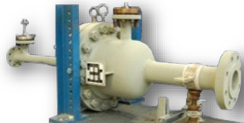
5 MWth Natural Gas CPOX
